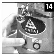
Moving quickly, turn off the Heat. Then, turn on the vacuum using the "Model" switch, and...
