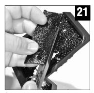
Cut excess plastic sheet from the vacuum formed part.
