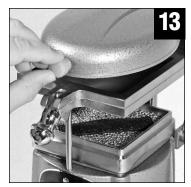
Grab the heater knob (do not touch the metal part of the machine – it gets HOT!). Swing the heater over the center of the plastic sheet and watch for the plastic to soften and sag down in the frame about 3/4". Experiment with different amounts of sag for different plastics; your experience will help judge when to do the next step.
