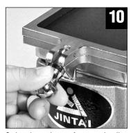
Swing down the top frame and pull the latch knob over the tongue to lock it in place. This will clamp the two frames together and hold the plastic ready for heating and forming.
