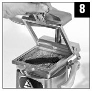
Swing up the top half of the frame. It should stay in place. If the frame does not stay up, tighten the two screws at the left and right rear supporting hinges a bit.
