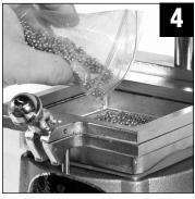
Optional – Pour the metal beads into the vacuum chamber. The beads act as a way to support patterns with irregular bottoms. If your pattern has a smooth bottom, you may elect to skip this step.
