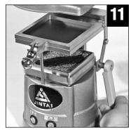
Push the orange handle down to latch the metal frame in the UP position.
