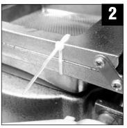
After removing the plastic tie(s) that hold the frame together for transport safety, you will notice either a piece of black plastic or wood inside the frame that is also for transport only and needs to be removed as well prior to operation.
