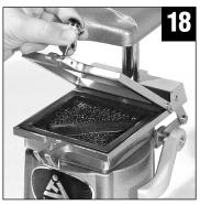
Unlock the frame and swing up the top half.
