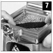
Use your fingers to push the metal beads around the bottom perimeter of your pattern. This will keep the plastic from wrapping around the pattern, making it difficult to remove later in the process.
