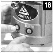
After about 8 seconds (to allow the plastic to cool), turn off the vacuum.
