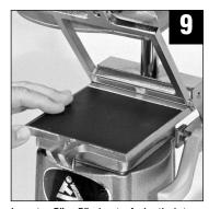
Insert a 5" x 5" sheet of plastic into the recess in the bottom frame.
