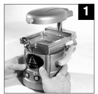
Unpack the machine and place it on your workbench in the position shown. Notice that the orange handle is in the horizontal position and the two control switches on the front of the machine are in the OFF position. Plug the line cord into a wall outlet. Note: The heater draws a lot of current, so try to avoid using an extension cord that could overheat.
